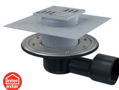
APV3344 Floor drain 105×105/50/75 mm side outlet, stainless steel grid, stainless steel flange and collar-2nd level insulation, wet and dry odour trap
