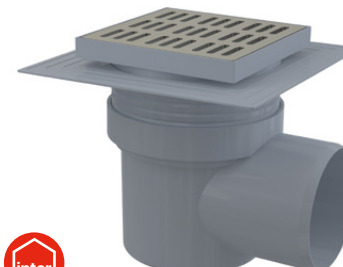
APV12 Floor drain 150×150/110 mm side outlet, stainless steel grid, collar-2nd level insulation, wet odour trap
