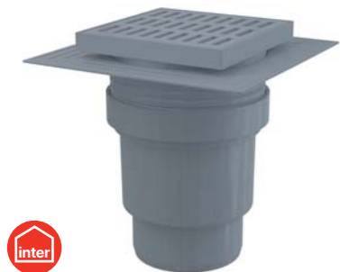
APV11 Floor drain 150×150/110 mm straight outlet, grey grid, collar-2nd level insulation, wet odour trap
