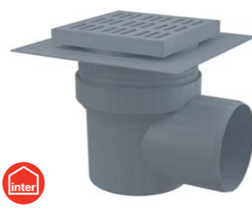
APV10 Floor drain 150×150/110 mm side outlet, grey grid, collar-2nd level insulation, wet odour trap
