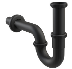
A4320BLACK Wash-basin trap "U" DN32, with coupling nut 5/4", black-matt
