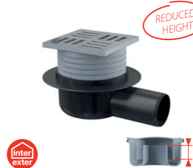
APV26 Floor drain 105×105/50 mm side outlet, stainless steel grid, wet odour trap
