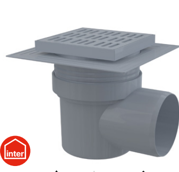
APV10 Floor drain 150×150/110 mm side outlet, grey grid, collar-2nd level insulation, wet odour trap
