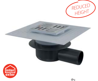
APV26C Floor drain 105×105/50 mm side outlet, stainless steel grid, collar-2nd level insulation, dry odour trap
