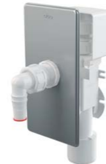
APS3P Concealed washing machine trap with air-admittance valve, stainless steel DN40 and DN50
