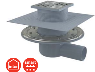
APV1324 Floor drain 105×105/50 mm side outlet, stainless steel grid, stainless steel flange and collar-2nd level insulation, combined odour trap SMART
