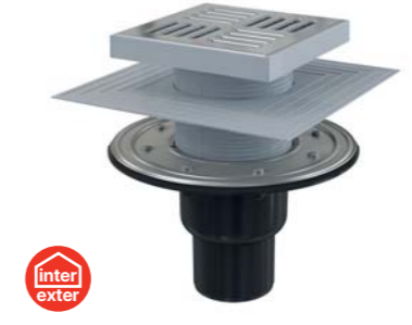
APV4444 Floor drain 150×150/50/75 mm straight outlet, stainless steel grid, stainless steel flange and collar-2nd level insulation, wet and dry odour trap
