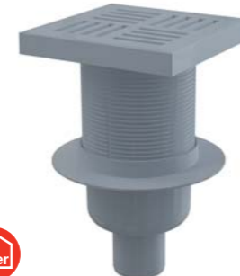
APV6211 Floor drain 150×150/50 mm straight outlet, grey grid, wet odour trap
