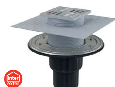
APV4344 Floor drain 105×105/50/75 mm straight outlet, stainless steel grid, stainless steel flange and collar-2nd level insulation, wet and dry odour trap
